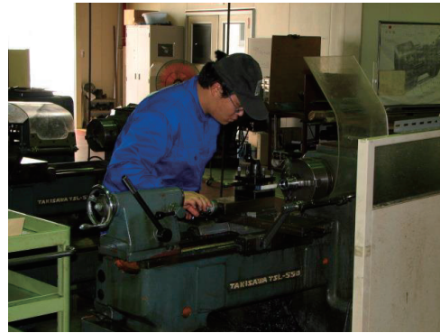
Fig. 3: Machining experience such as contour cutting and end face cutting using Engine lathe
