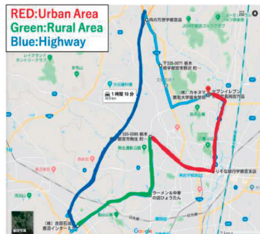
Fig. 1 Real Driving Road Test in Utsunomiya City
